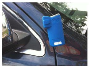
Magnets on both sides of the instrument strongly adhere to ferrous metal surfaces such as a car, to prevent instrument loss during the heat of an arrest.
